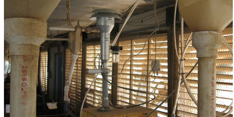
Researchers have positioned a sampling port and instruments in front of the primary exhaust fan in this building to measure exhaust gases, particulates, temperature, and relative humidity. Photo by Ken Casey.
